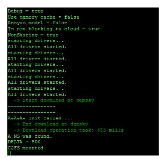
Figure 94 - mounting and sync of DepSky driver with remote buckets
